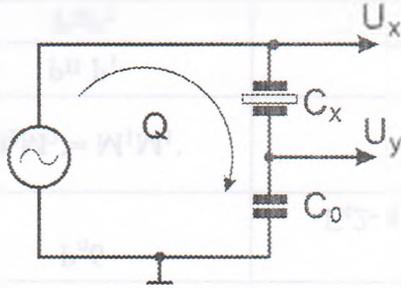
Figure 2. Schematic diagram of dielectric hysteresis loop measurement.
