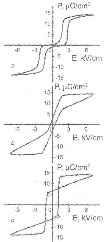
Figure 10. Measured dielectric hysteresis loops of  $\text{Sn}_2\text{P}_2\text{S}_6$  crystal at room temperature and 10 Hz switching field frequency and different ratios of ferroelectric and antiferroelectric regions in the crystal volume..
