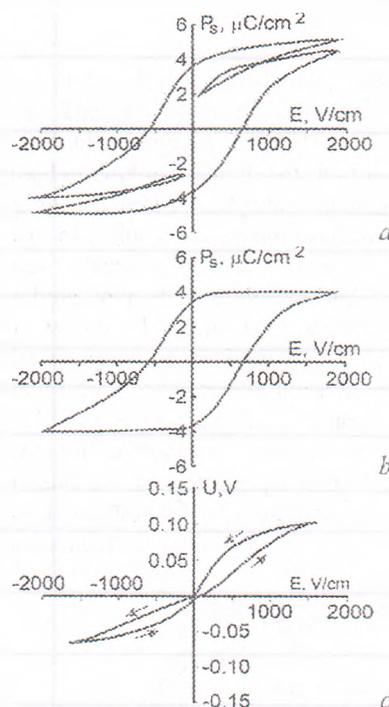
Figure 6. Measured (a) and reconstructed (b) dielectric hysteresis loop of  $\text{Sn}_2\text{P}_2\text{S}_6$  crystal at room temperature and 10 Hz switching field frequency. (c) Voltage dependence on the reference capacitor  $C_0$  ( $2.2 \mu\text{F}$ ). Arrows show the course of the applied voltage change.
