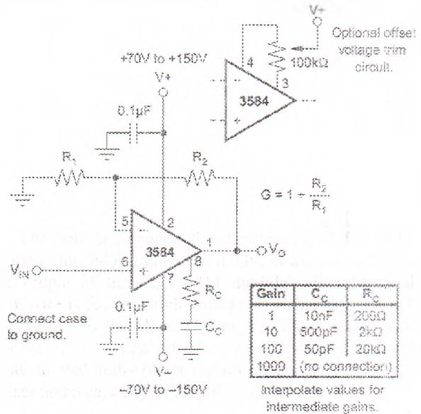
Figure 8. Schematic diagram of a high-voltage amplifier [13].
