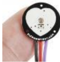
Fig. 4. Removing the signal from the sensor "Pulse Sensor" (when the signal is removed, the sensor is turned back to the fingertip).
